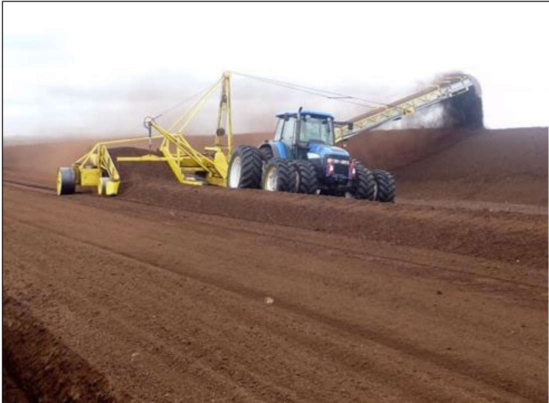
Plate 4-12: Harvesting – Peco method. Image: Bord na Móna
