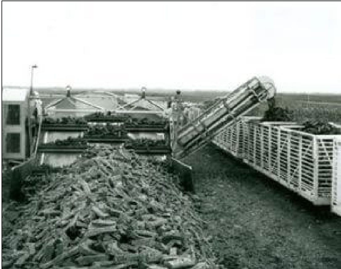
Plate 4-23: Sod Peat Loading Machine. (Source: https://www.bordnamonalivinghistory.ie/equipment-detail/loading-machine/ )
