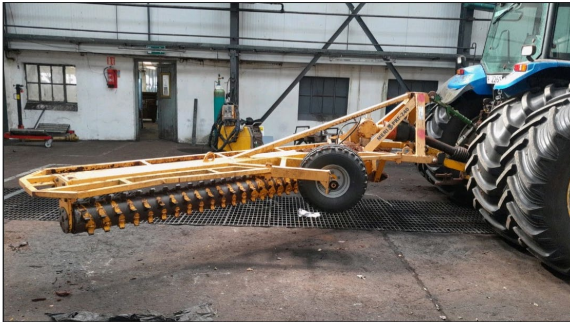
Plate 4-28: Offset (Type-I) Miller attachment. (Source: Bord na Móna site personnel)
