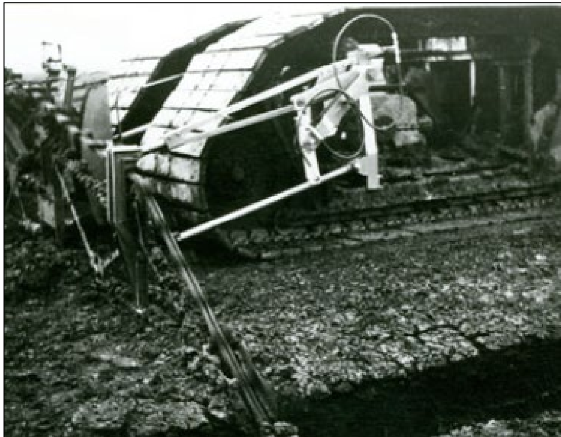
Plate 4-4: Drain Cutting Attachment – Cross Drain. Source: https://www.bordnamonalivinghistory.ie/equipment-detail/drain-cutting-attachment-cross-drain/
