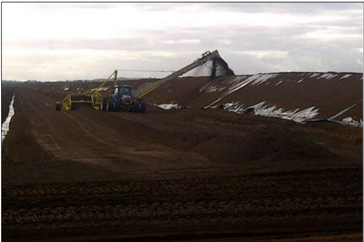
Plate 4-15: Process of Stock Protection, showing a layer of milled peat being spread over polythene sheeting to anchor the sheeting in place (source: Bord na Móna)
