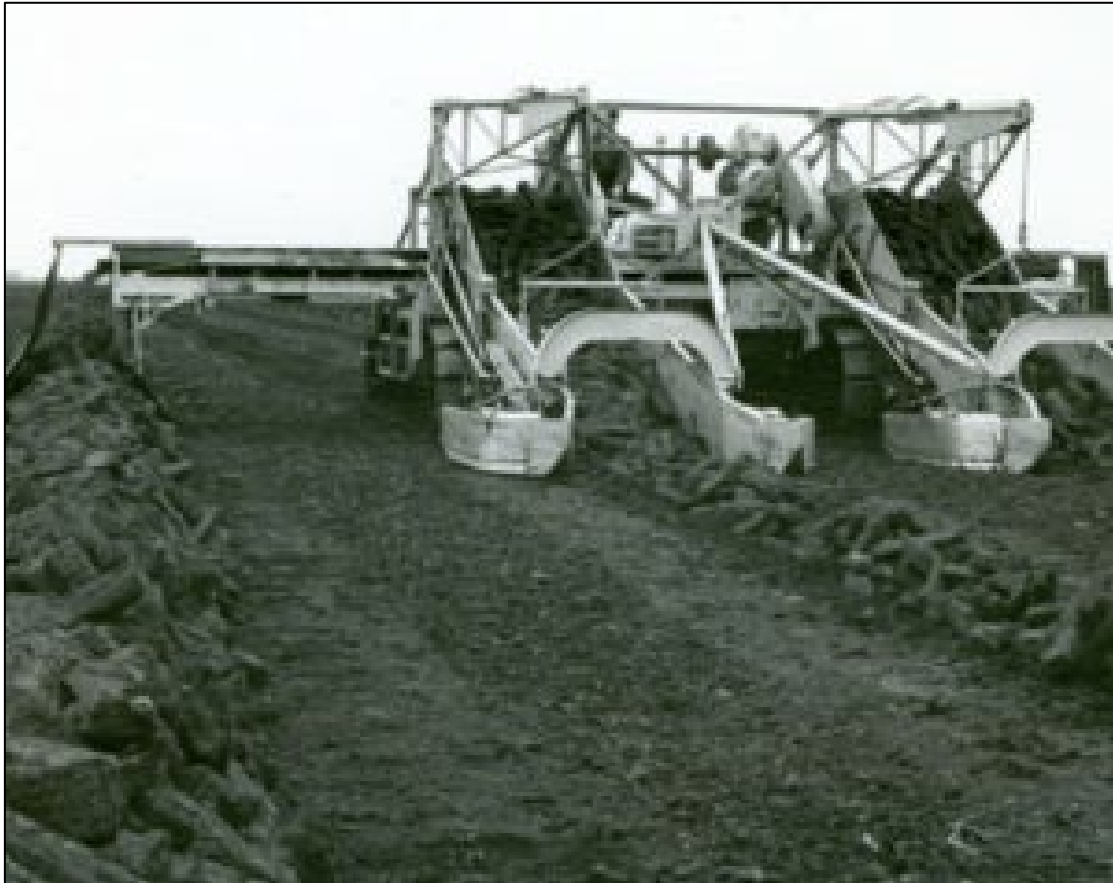
Plate 4-19: Sod turning machine. (Source: https://www.bordnamonalivinghistory.ie/equipment-detail/sod-turning-machine/ )
