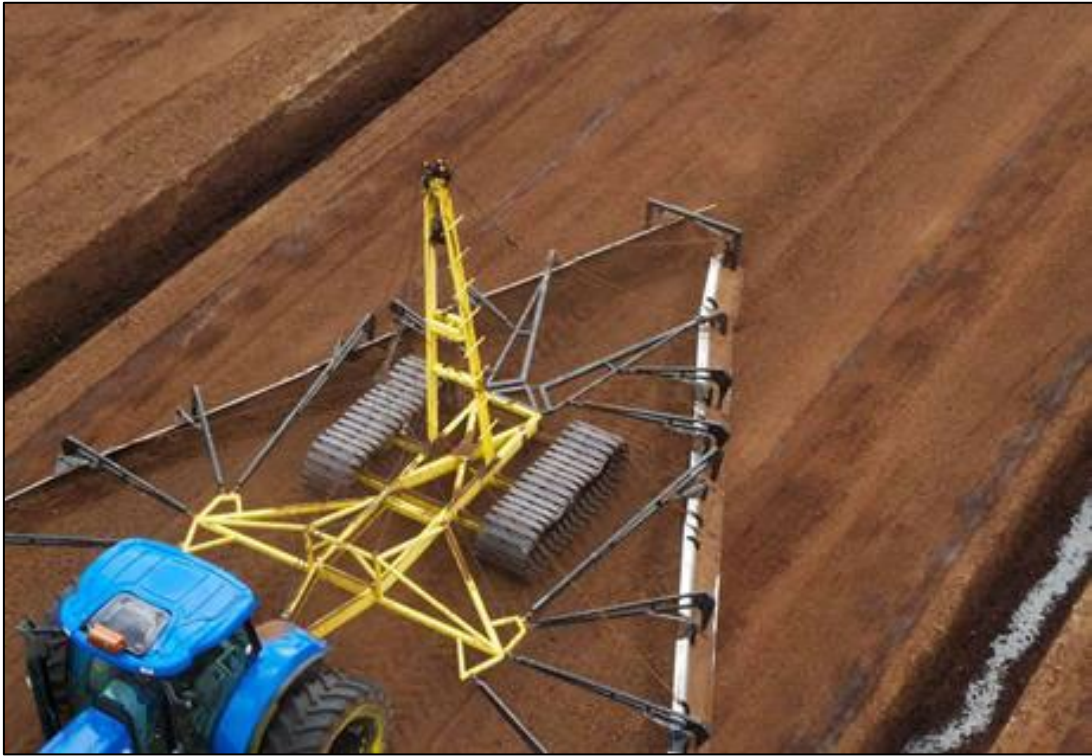
Plate 4-10: Ridging process. Image: Bord na Móna
