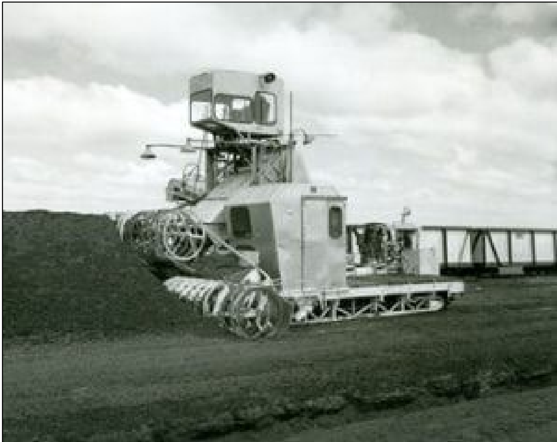
Plate 4-31: Milled Peat Loading Machine. (Source: https://www.bordnamonalivinghistory.ie/equipment-detail/loading-machine/ )
