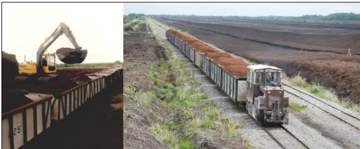
Plate 4-35: Example of railway locomotive and wagons hauling milled peat to the power plant (source: Bord na Móna)
