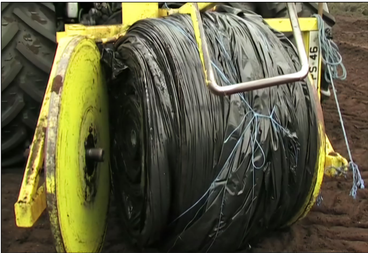
Plate 4-33: Polywrapper with the frame opened to allow access to the collected bale of polythene
