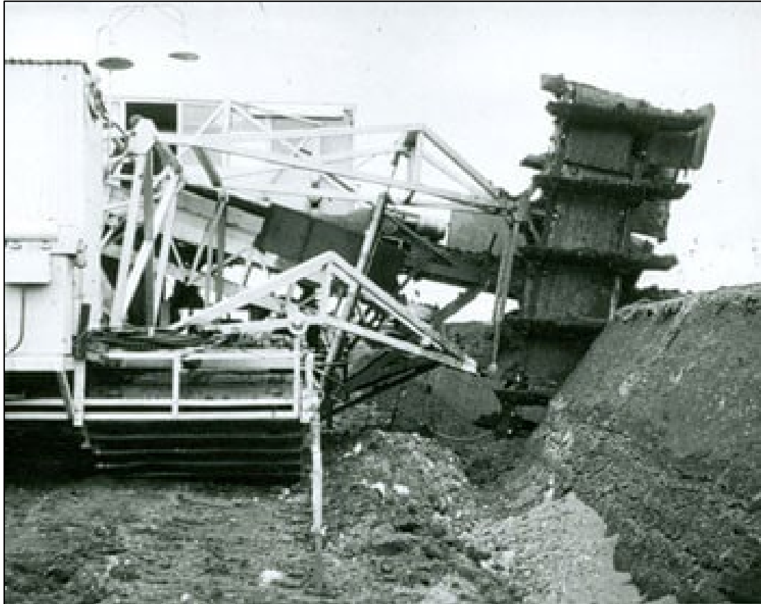
Plate 4-22: Cutaway Boom Attachment. (Source: https://www.bordnamonalivinghistory.ie/equipment-detail/cutaway-boom-attachment/ )
