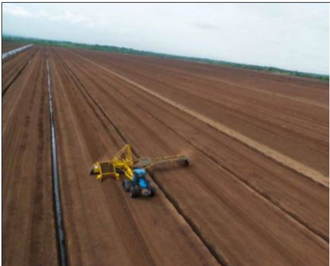
Plate 4-13: Harvesting – Peco method. Image: Bord na Móna
